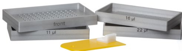
Resin dispenser set for dispensing resin in to the tip reactors.
