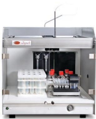
Syro I (one robot arm and one reactor block)
