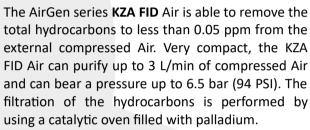
The reduction of hydrocarbons, including methane, and carbon monoxide decrease the background noise level and gives much better baseline stability, considerably increasing detector sensitivity and ensuring precise analytical results. High efficiency coalescing pre-filtration and post filtration of particulate size greater than 0.01 microns are used to prevent any kind of particles from entering the analytical device.
