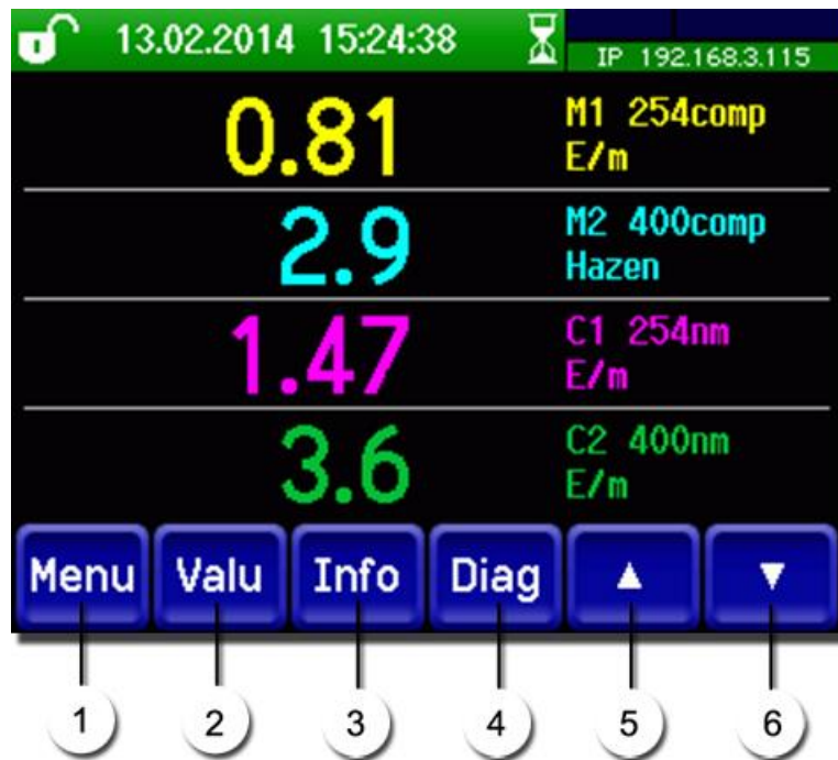
Figure 12: Control elements in measuring mode
