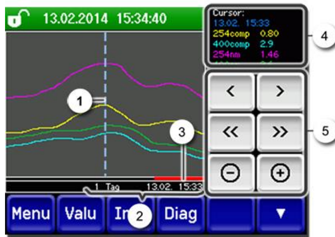
Figure 16: Functions of the Log display
